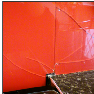
Untoughened glass always cracks when broken
